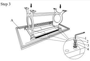
Notes : -Attached complete Leg Frame to Table Top. -Fully tighten the bolt.
